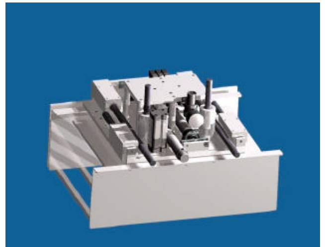
Gripper for inconsistent bags
