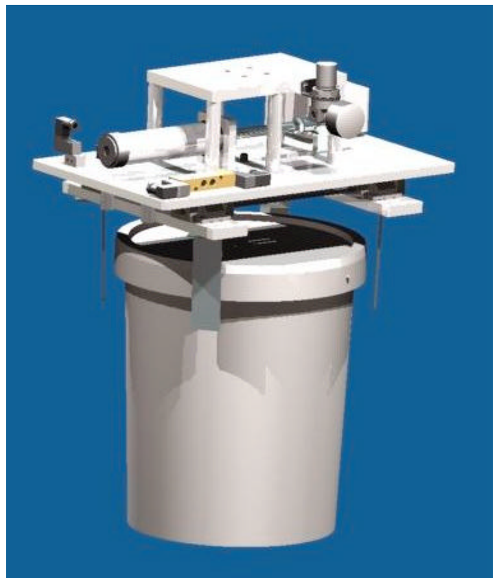
Self-centering gripper with hooks for buckets
