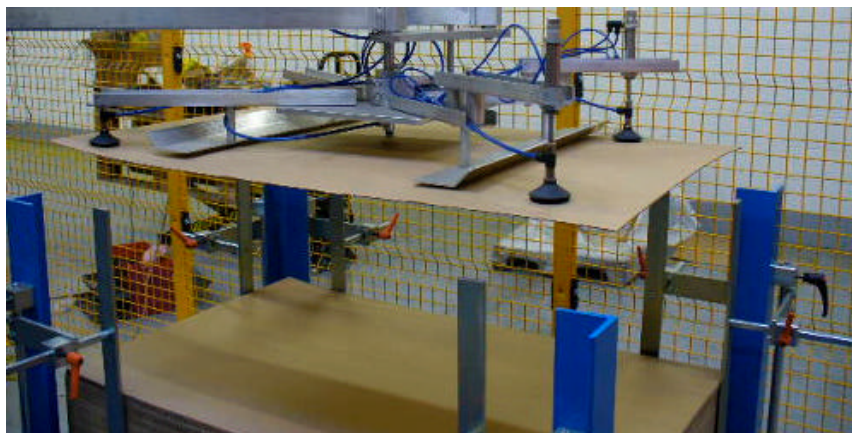
Gripping element with suction cups
